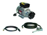
For oil transfer - 40 lt/min. Self-priming, rotary, vane pump, with protection class IP55 and by-pass valve. For diesel and oil, with rubber exit hose (4 mt), aluminium gun, rubber tail pipe with filter. Max pressure 2-3 bar. Maximum output 70 It/min.
